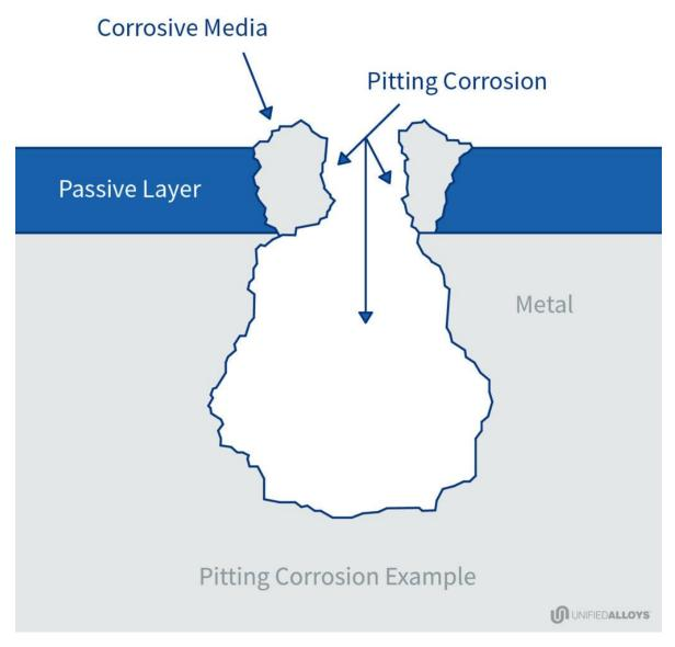
Pitting corrosion occurs on metals with protective films — such as stainless steel.
